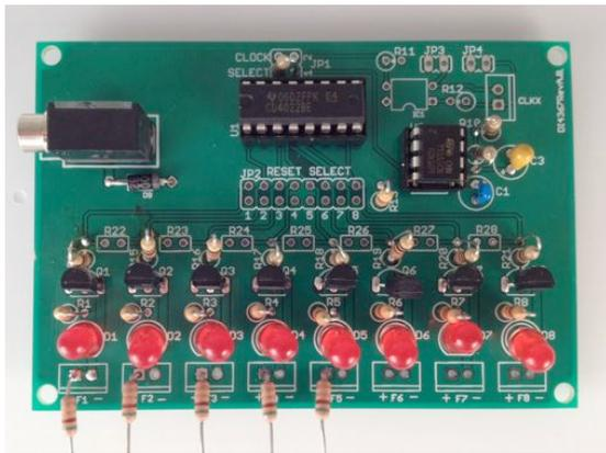
Fig. 4.1: PCB populated with supplied components.
