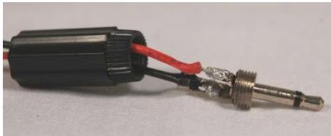
**Fig. 5.2:** Wiring to plug. Mini jack soldered to battery pack.
